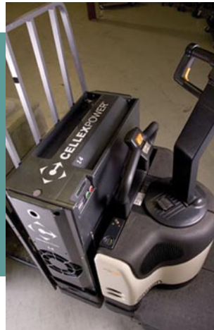
Cellex's CX-P150 fuel cell power unit in a rider pallet truck and being fueled. Photos courtesy of Cellex Power Products, Inc.
